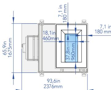
Inspection hatch: required close to the projector.
