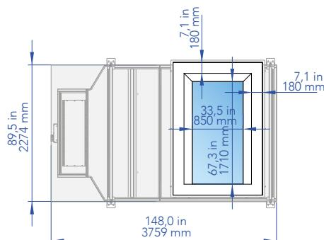
Inspection hatch: required close to the projector.
