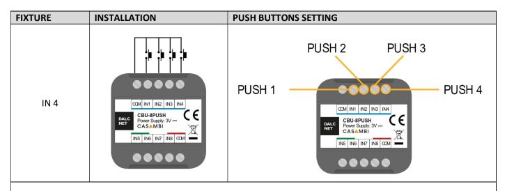
With this fixture it is possible to configure up to 4 N.O. push buttons. Each push button can control a luminaire, control a group of luminaires, control a scene or an animation. This configuration is possible to set by Casambi APP.
