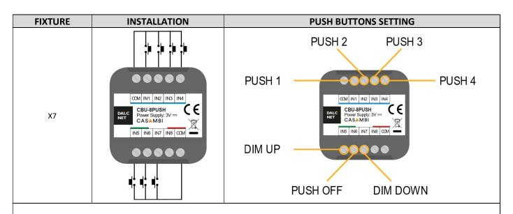
With this fixture it is possible to set up maximum 4 N.O. push buttons. Each push button can control a luminaire, control a group of luminaires, control a scene or an animation. This configuration is possible to set by Casambi APP.
